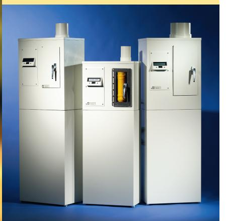
The Eagle Pneumatic Mark II Air-Lift System, a durable and supremely reliable pressure/ vacuum system, requires power only at one end of the system. Located at either end of the system, the send/receive station is called the "power pedestal." The system moves carriers in one direction using pressure and with vacuum power on return, resulting in a highly dependable "push-pull" system operation.
